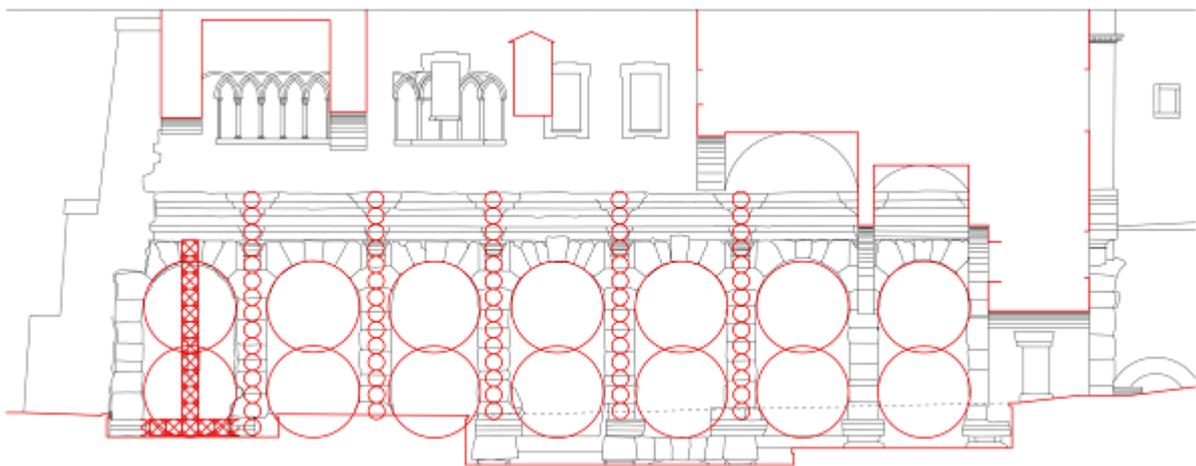
*Fig. 2 Tempio di Claudio in Rome. Geometric longitudinal section. Inserted are schemes showing the proportions*
