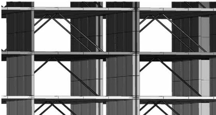
Figure 8 Wind bracing tension rod scheme
