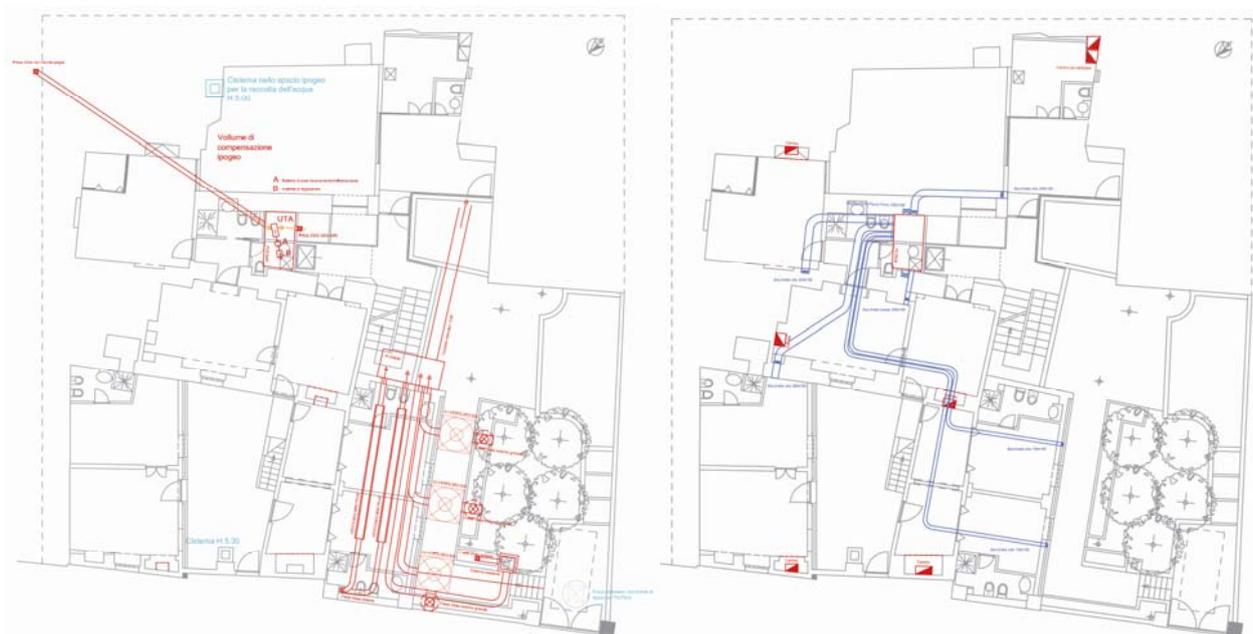
Figure 7. On the left: Ground Floor Plan, natural intake system and passive air treatment. On the right: First Floor Plan, air distribution and extraction system.
